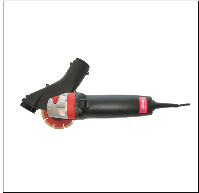
TNO reference 125 mm angle grinder, model Metabo WE 9-125 Quick, with TNO/Dusttool dust shroud.
