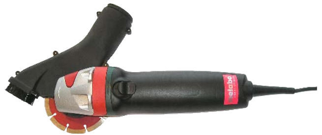
TNO Reference 125 mm angle grinder (type WE 9-125 Quick) with Dusttool extraction hood
